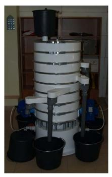
Fig. 2. A rolling-screw screen with a fraction receiver (Pocwiardowski and Wodzinski 2011b)
