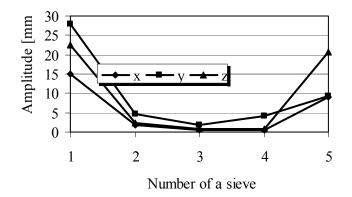
Fig. 8. Sieves oscillation amplitude within X , Y , Z axis with the motor-vibrators inclination angle of  $45^{\circ}$
