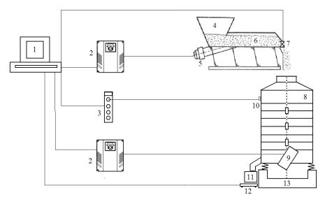
Fig. 9. The mechatronics system diagram
