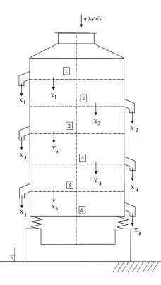
Fig. 1. The diagram of the screening process using a rolling-screw screen
